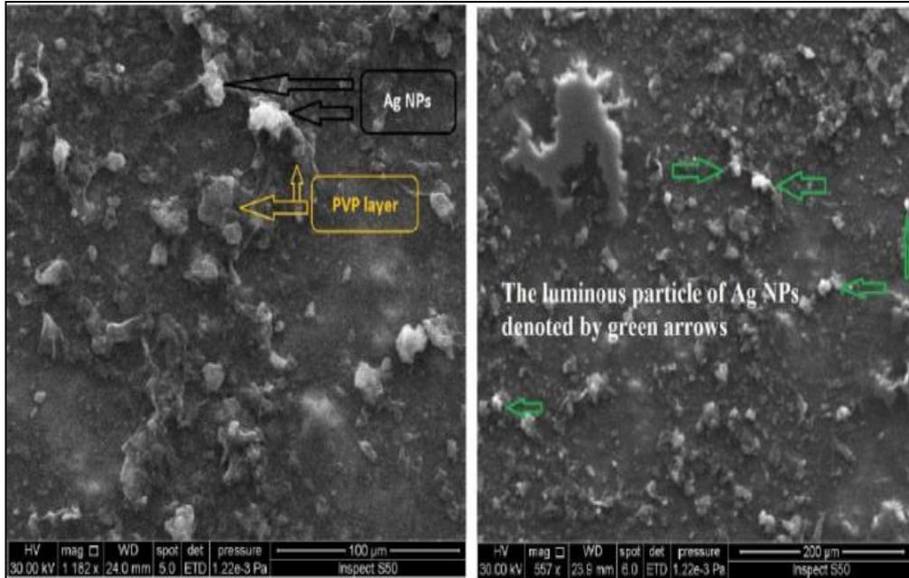
**Fig. 3.** SEM images of the PVP capped with the film silver NPs.
