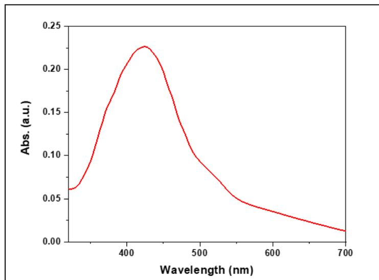
**Fig.5.** Absorption peak of silver NP<sub>a</sub> ( $\lambda = 410$  nm).
