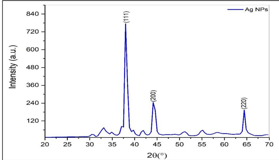
**Fig. 1.** The pattern of XRD of the Nanoparticles.
