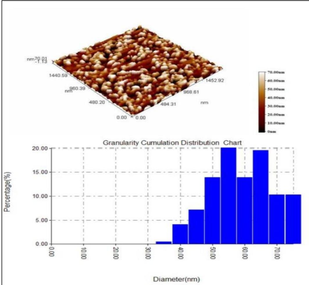
**Fig. 2.** The AFM image for Ag NPs / PVP.
