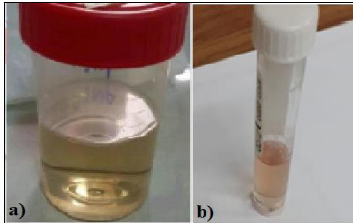
**Fig. 9.** Color of silver NPs colloids when pH is: a) pH = 11, b) pH = 5.
