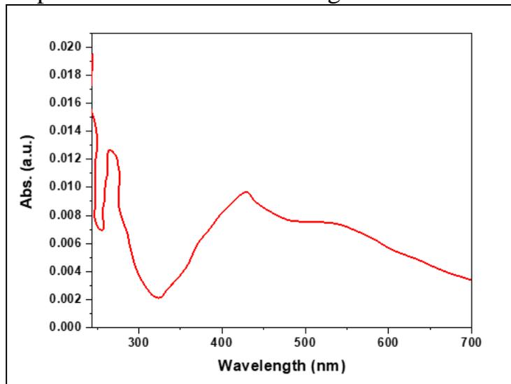
**Fig.4.** Absorption peak of silver NPs ( $\lambda = 426$  nm).
