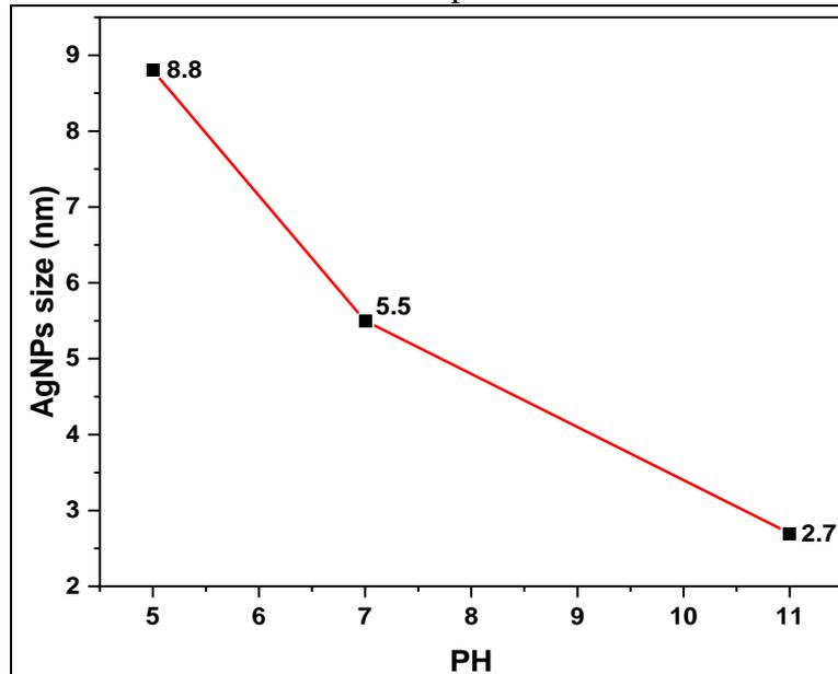
Fig. 8. Relationship of the values of the pH versus size of silver NPs.
