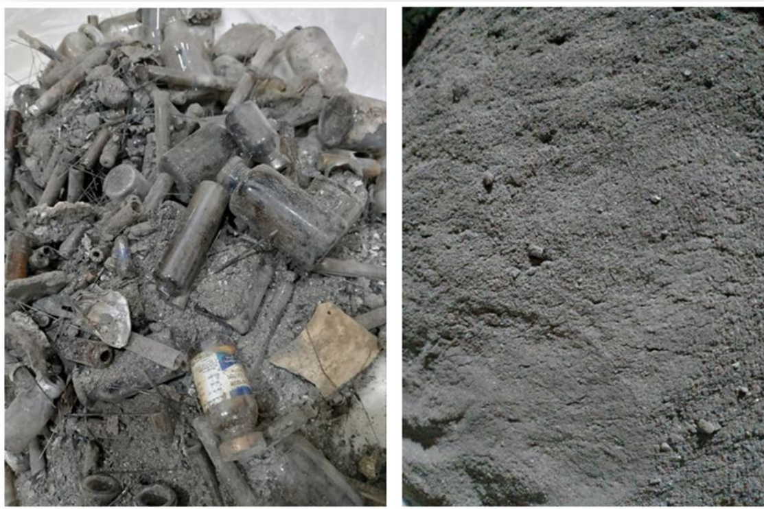
Figure 2. Medical waste ash before and after the grinding process
