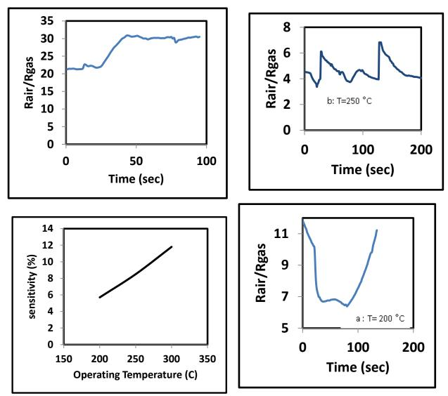
Figure (3): The sample (1) gas sensor response at 6 volt bias voltage and operating temperature ((a) 200, 250 (b) and 300 (c)) <sup>o</sup>C, (d) sensitivity vs. operating temperature.
