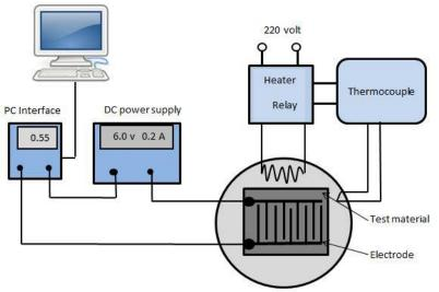
Figure (2): scheme of the used gas sensor testing setup.
