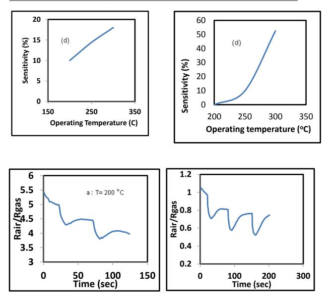
Figure (6): The sample (4) gas sensor response at 6 volt bias voltage and operating temperature ((a) 200, 250 (b) and 300 (c)) <sup>o</sup>C, (d) sensitivity vs. operating temperature.
