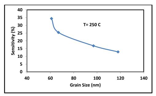
Figure (7): The sensitivity vs. sample grain size at operating temperature T = 250 °C.
