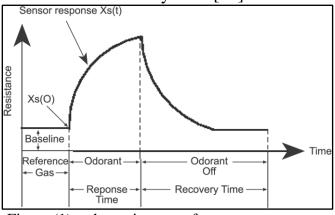
Figure (1): schematic trace of gas sensor response
