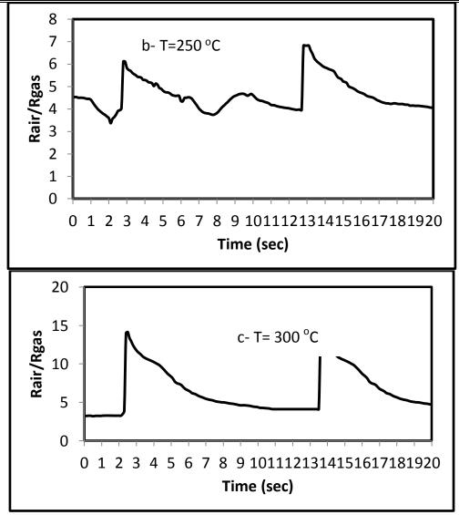
Figure (3): The gas sensor (of  $t_1$ =102.69 nm) response at 6 volt bias voltage and operating temperature ((a) 200, 250 (b) and 300 (c)) °C.
