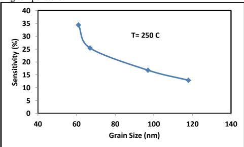
Figure (5): The sensitivity vs. sample grain size at operating temperature T = 250 °C.
