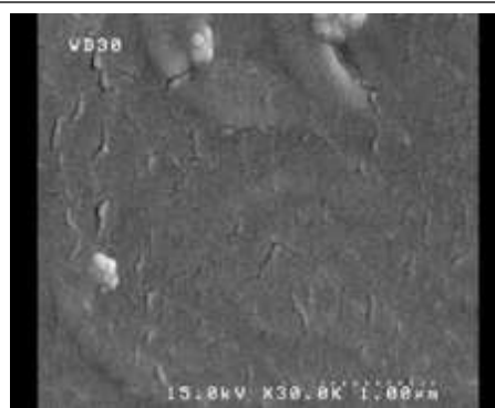
Fig. ( 16). Ttopography of fractured structure of EP// ZrO_2 nanocomposites (4 % vol. fraction of/ ZrO_2 ).
