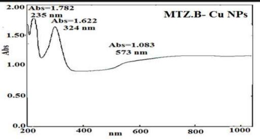
Figure 4 b - The UV-Visible spectra of antibiotic MTZ.B  $(3.6 \times 10^{-4} \text{ M})$  and MTZ.B Conjugation Cu NPs in aqueous solutions at room temperature using (copper (II) sulphate salt solution), pvp, ascorbic acid and MTZ.B  $(0.2, 10.8 \times 10^{-3}, 0.289 \text{ and } 3.6 \times 10^{-4} \text{ M}$  respectively) at pH 7 after 1 h.
