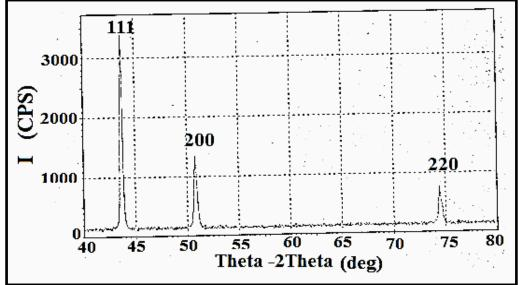
Figure 6 - The XRD pattern of the MTZ.B –capped copper NPs using (copper (II) sulphate salt solution, pvp, ascorbic acid and MTZ.B (0.2,  $10.8 \times 10^{-3}$ , 0.289 and  $3.6 \times 10^{-4}$  M respectively) at pH 7
