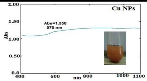
Figure 4 a - The UV-Visible spectra of  $CuSO_4$  .5H<sub>2</sub>O (2x10<sup>-2</sup> M), L-ascorbic acid, Cu NPs and their images in aqueous solution using (copper (II) sulphate solution, pvp (Mw nearly 10 000), and ascorbic acid (0.2M, 10.8 x 10<sup>-3</sup> M, and 0.289M, respectively) at pH 7 after 30 minutes.
