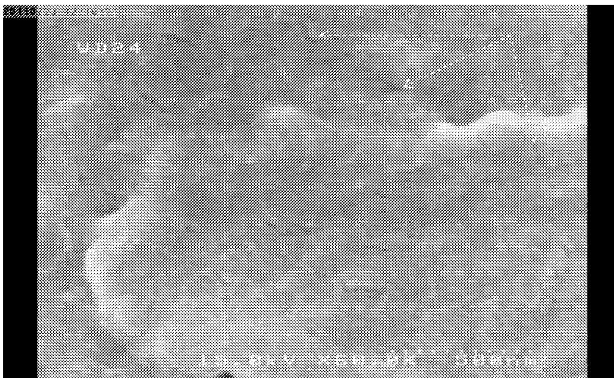
Fig. ( 3E). Fracture structure topography of nanocomposies (EP/ 4 vol.% nano SiO 2 ).
