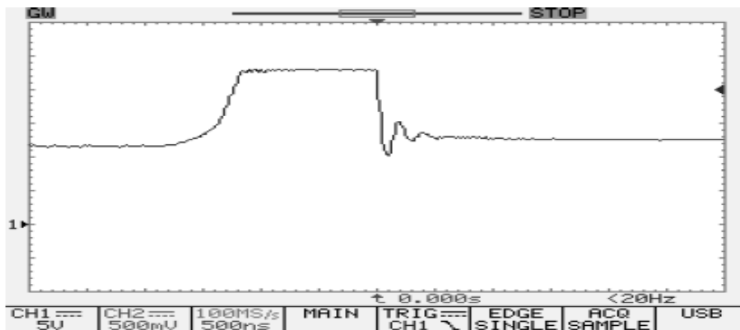
Fig.( ١٠ ) Slave module MOSFET Avalanche waveform, ٢٣V peak.
