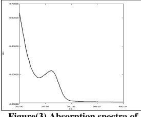
Figure(3) Absorption spectra of 12 µg/ mL Cephalexine
