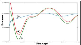
Figure No. (7) first derivatives spectra of (a) 12  $\mu$ g/mL Cephalexin , (b) 12  $\mu$ g/mL Cefixime (c) Cefixime and Cephalexin
