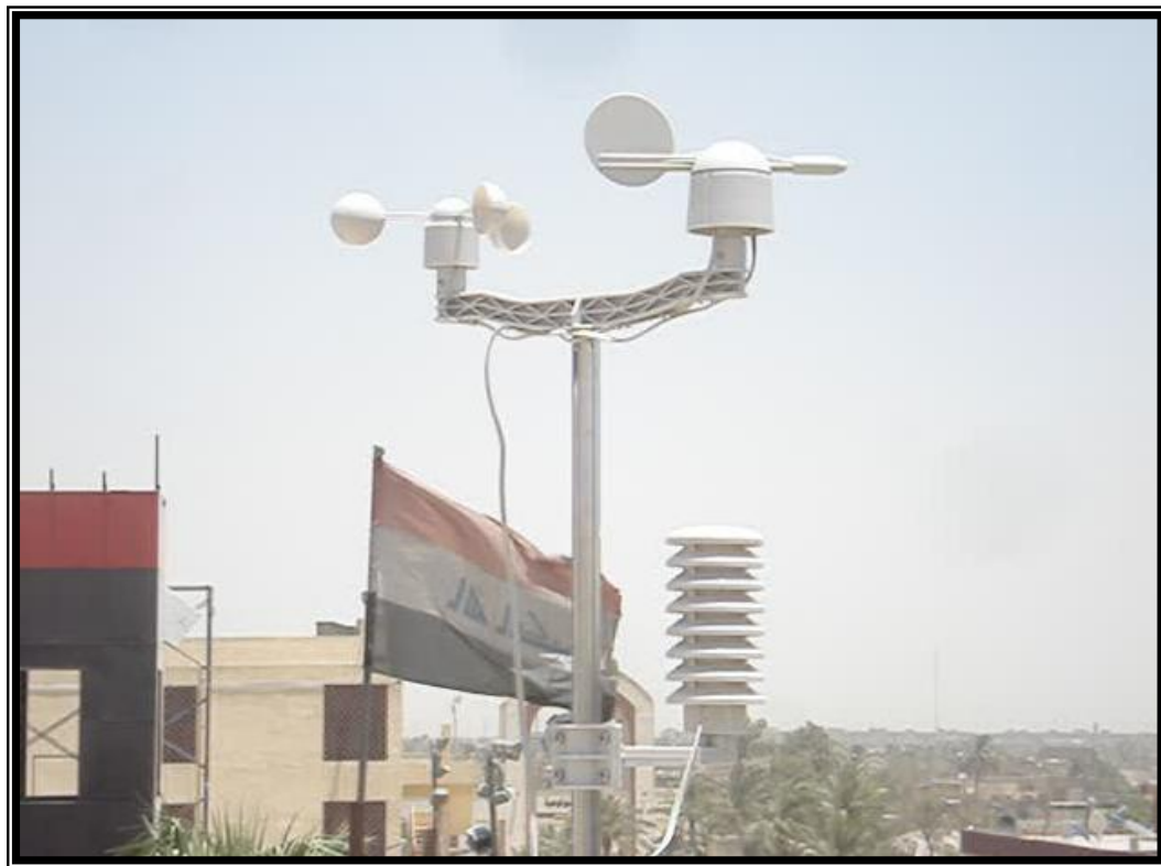
Fig. 8 Illustrate unit sensors of the proposed weather system
