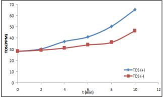
**Figure 7** -The effect of corona discharge on TDS - time relationship of the distilled water in positive corona (blue line) and negative corona (red line).
