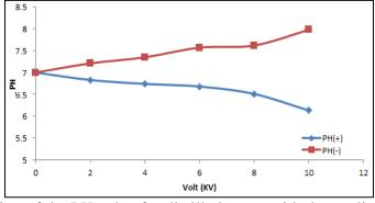
**Figure 3 -** Variation of the PH value for distilled water with the applied voltage of both positive (blue line) and negative (red line) corona discharges.
