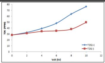
**Figure 4** -Variation of TDS for distilled water versus the applied voltage of both positive (blue line) and negative (red line) corona discharges.
