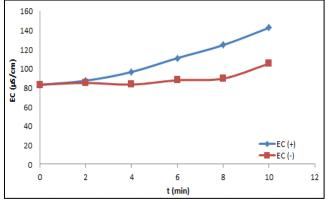
**Figure 8 -** The effect of corona discharge on EC - time relationship of the distilled water in positive corona (blue line) and negative corona (red line).
