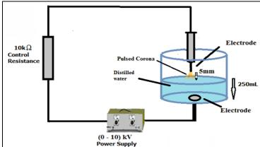
Figure 1 - Schematic diagram of the electrical discharge system.
