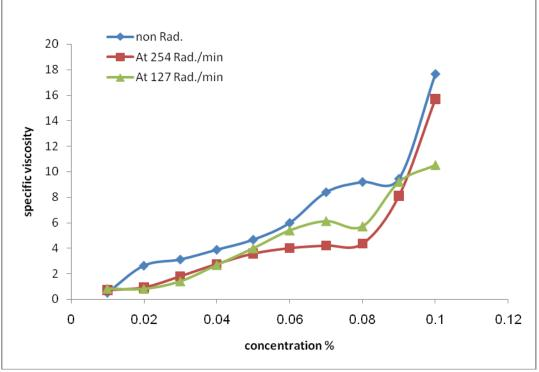
Figure 3: Specific viscosity changed with concentration for PAAM in Ethylene glycol.
