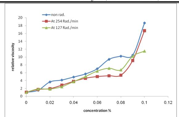
Figure 2: Relative viscosity changed with concentration for PAAM in Ethyleneglycol.
