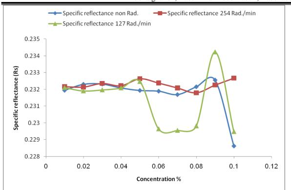
Figure 10: Specific reflectance of polyacrylamide in ethylene glycol at different concentration before and after radiation.
