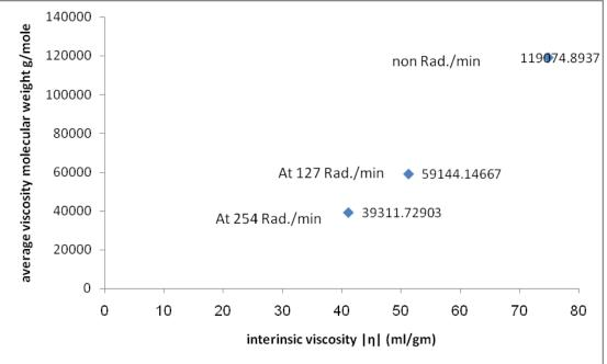
Figure 5: Average viscosity molecular weight of polyacrylamide before and after Radiation.
