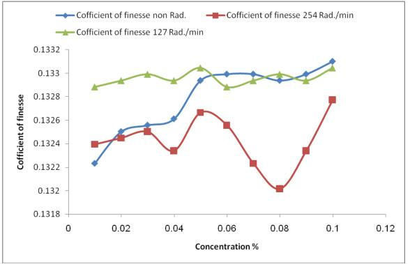
Figure 9: Coefficient of finesse of polyacrylamide in ethylene glycol at different concentration before and after radiation.
