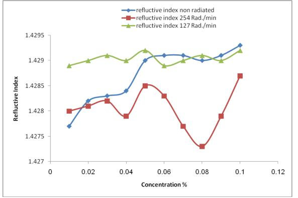
Figure 7: Reflective index of polyacrylamide in ethylene glycol at different concentration before and after radiation.
