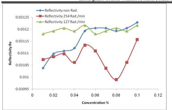
Figure 8: Reflectivity of polyacrylamide in ethylene glycol at different concentration before and after radiation.
