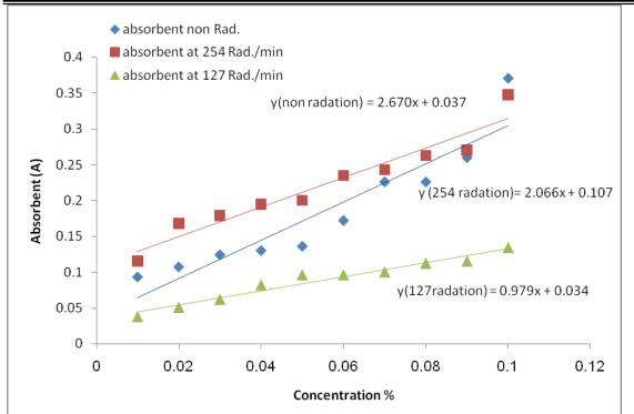
Figure 6: absorbent of polyacrylamide in ethylene glycol at different concentration before and after radiation.
