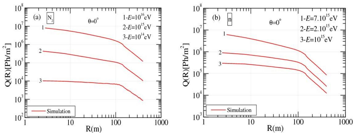
**Figure 2.** Lateral distribution of Cherenkov light which simulated with CORSIKA code for (a) primary Nitrogen at the energies 10<sup>14</sup>, 10<sup>15</sup> and 10<sup>16</sup> eV for vertical showers; (b) primary Neutron at the energies 10<sup>15</sup>, 2.10<sup>15</sup> and 7.10<sup>15</sup> eV for vertical showers.
