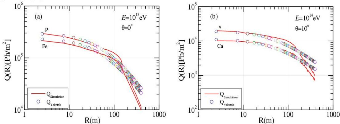
**Figure 6.** Lateral distribution of Cherenkov light which is simulated with CORSIKA code (solid lines) and one measured with Yakutsk array (symbol lines) for (a) primary proton and iron nuclei for vertical shower at energy  $10^{15}$  eV; (b) primary neutron and calcium for angle  $\theta = 10^\circ$  at energy  $10^{16}$  eV.
