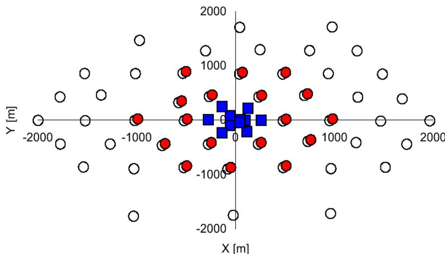
Figure 1. The detector arrangement of the Yakutsk Array [3].
