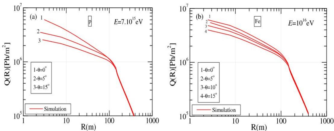
**Figure 3.** Lateral distribution of Cherenkov light which simulated with CORSIKA code for (a) primary proton at the energy 7.10<sup>15</sup> eV and different angles  $\theta = 0^\circ, 5^\circ$  and  $15^\circ$ ; (b) iron nuclei at the energy 10<sup>16</sup> eV and different angles  $\theta = 0^\circ, 5^\circ, 10^\circ$  and  $15^\circ$ .
