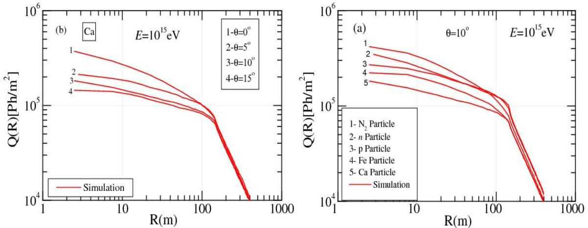
**Figure 4.** The lateral distribution function of Cherenkov light simulated by CORSIKA code at the energy  $10^{15}$  eV for; (a) Nitrogen, Neutron, proton, iron nuclei and Calcium particles at  $\theta=10^\circ$  and (b) primary Calcium for different angles  $\theta=0^\circ, 5^\circ, 10^\circ$  and  $15^\circ$ .
