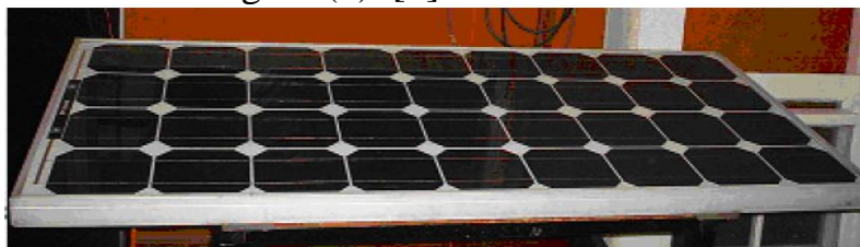
Figure (3) monocrystalline photovoltaic module.
