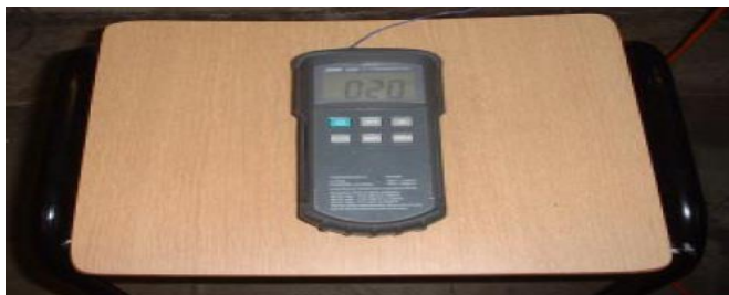
Fig.(5 ) Thermometer. The range (-50 °c to 1300 °c)
