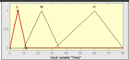
Fig. (7) Membership function of Temperature Temp.
