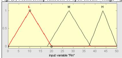
Fig. (6) Membership function of incident power density P<sub>in</sub>
