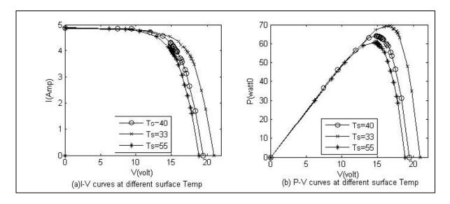
Fig. (1) a I-V curves at different surface temperature. b P-V curves at different surface temperature.
