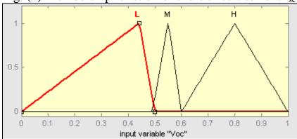
Fig. (5) Membership function of open circuit voltage V<sub>oc</sub>
