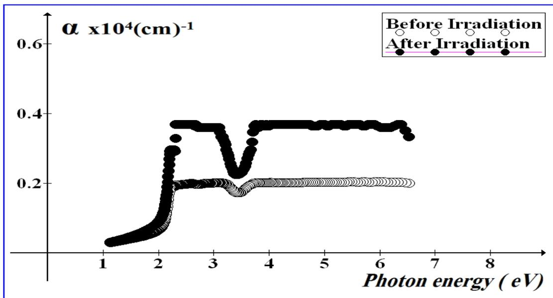
**Fig. (1) Absorption coefficient versus Wavelength(nm)**
