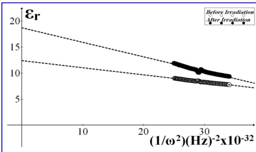
Fig.(3) Real dielectric constant vs. Reciprocal of square of angular frequency.
