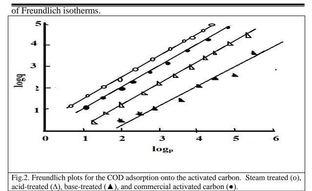
Loq q values represent the relative adsorption efficiency of the activated carbon, while logp represents the residual concentration of COD in the treated municipal wastewaters.
