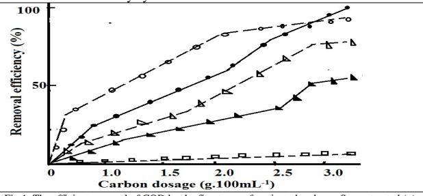
Fig.1. The efficient removal of COD by the five types of activated carbons. Steam treated (o), acid-treated ( $\Delta$ ), base-treated ( $\Delta$ ), heat-treated ( $\Box$ ) and commercial activated carbon ( $\bullet$ ).
