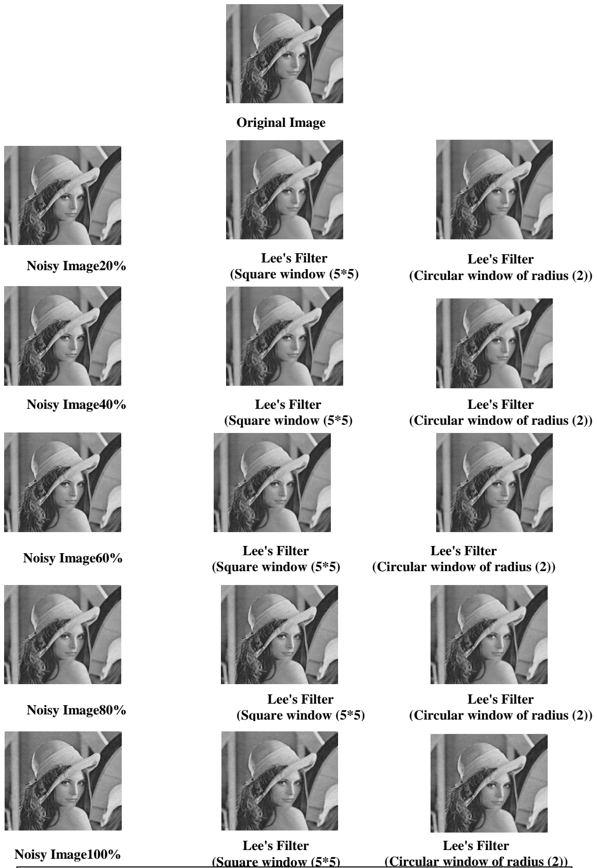
Fig. (3) Original, Noisy(additive Gaussian noise \sigma_n = 10 ) and smoothing images for Lena image
