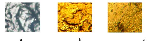
Figure 6. Shows the effect of thiourea concentrations on the grain structure of Ni-W alloy, a- no additives b- 5 g/l thiourea c- 10 g/l thiourea, T= 60  $^{\circ}$ C, j = 12 Adm<sup>2</sup> and with magnetic stirring.
