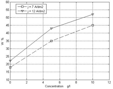
Figure 1. Shows the relation of W (weight percent )in the deposit with concentration of thiourea at PH=7, (j= 7 and 12  $A/dm^2$ ), T= 60 °C and with magnetic stirring.
