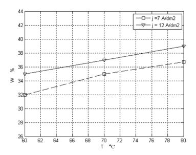
Figure 3. Shows the effect of the absence of magnetic stirring on the W( weight percent )at different temperature and current density with 5g/l thiourea.
