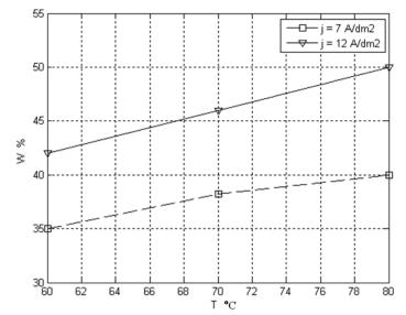
Figure 2. Describes the relation of temperature with W( weight percent )at different current density with magnetic stirring in 5g/l thiourea.
