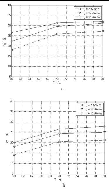
Figure 4. The relation of W content with temperature at different values of current density with no additives a- with stirring and b- without stirring.
