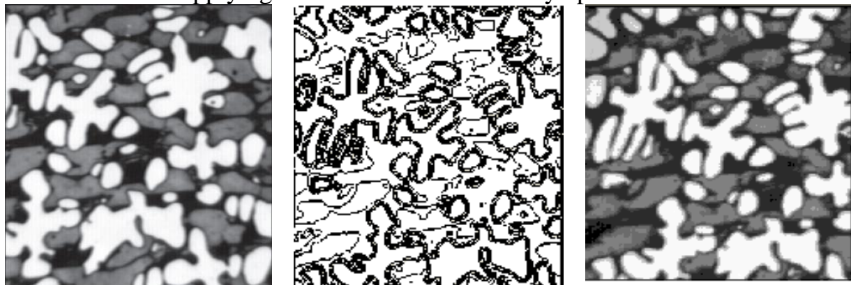
Fig(5) (a) microscope image (b) Threshold image (c) AND operation
